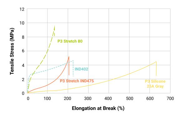
A stress-strain curve of Loctite 3D IND402 and P3 Stretch IND475 show their difference in physical behavior. Loctite 3D IND402 shows high initial resistance to stretching meaning it is more resilient and has more "springiness." P3 Stretch IND475 shows low resistance until breakage indicating it is a softer-touch material.
